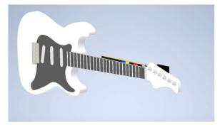
Modelling design two was far quicker. Again it was modelled in autodesk inventor and involed methods such as extrude, extruded cut and 3D sketch with a sweep to create the wire. The design housed the curcuits and battey behind the headstock, which leads to a shorter wire making for less disruption for the user.
