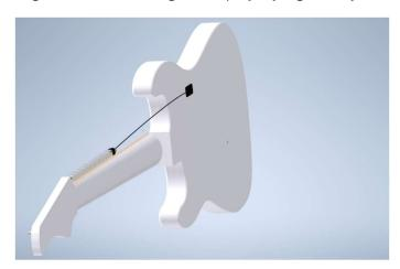
Design one used the 3D sketch tool in combonation with the sweep tool in order to create a wire from the final segment to the back of the guitar where the circuits and the battery are housed. When designing I chose to have the "brains" of the device at the back of the guitar to cause as little disruption to playing as possible.
